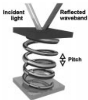
Figure 10. Scheme of a liquid crystal film.
